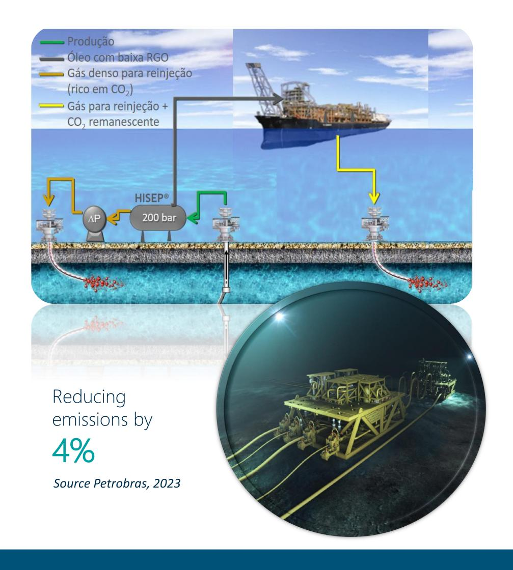
The high pressure CO2 separation technology (HISEP) is a solution that allows the gas leaving the reservoir to be separated and reinjected from a system located on the seabed.
