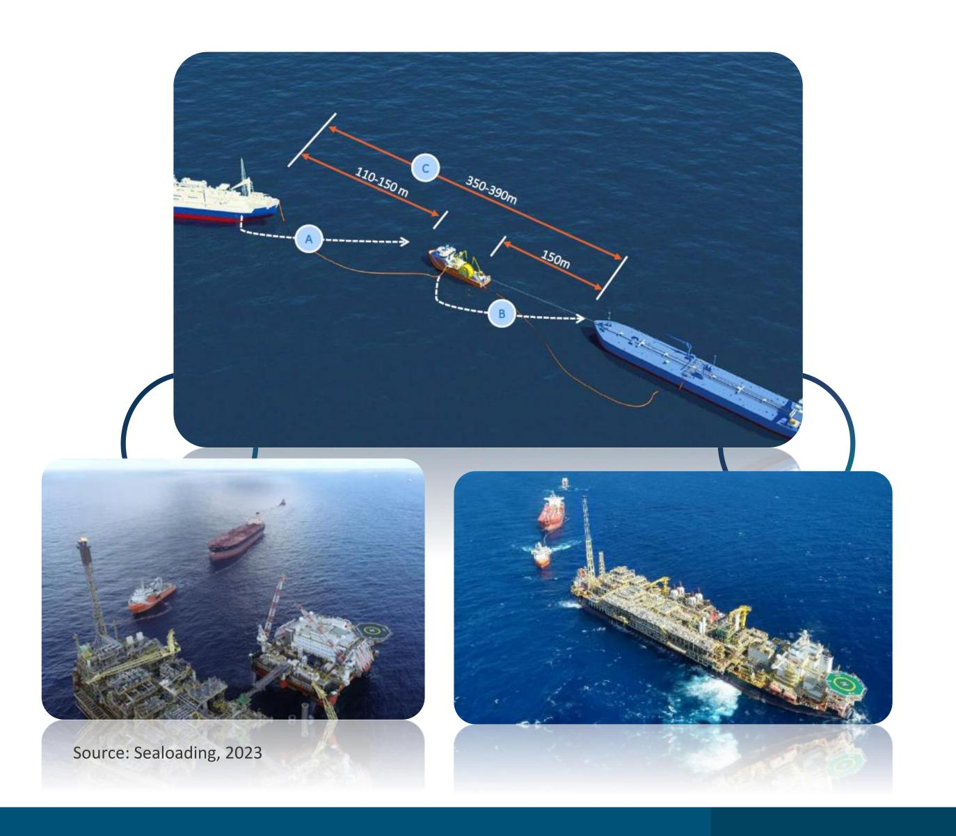
The CTV (cargo transfer vessel) technology is a cost efficient, flexible, safe and energy saving method of transferring oil from offshore oil fields onto conventional tankers.
